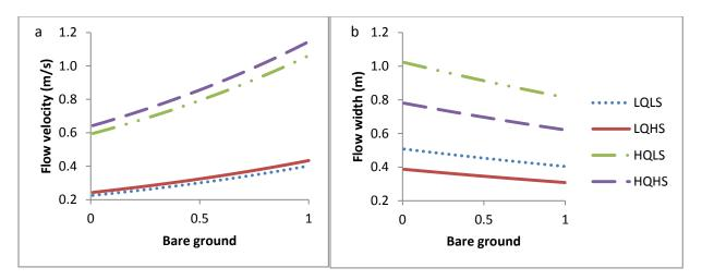
*Figure 6.* Flow velocity (a) and flow width (b) as a function of plot bare ground proportion using equations developed by (Al-Hamdan et al., 2012). High and low discharge rate (HQ, LQ) of 1L/s and 0.01 L/s were combined with steep and shallow slopes (HS, LS) of 1% and 40%.
