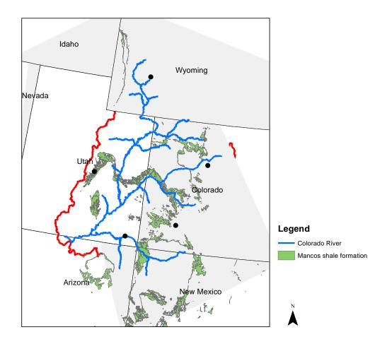
*Figure 9.* Map of the state of the UCRB highlighting Mancos Shale geologic formations contributing to most naturally occurring salt in the Colorado River.
